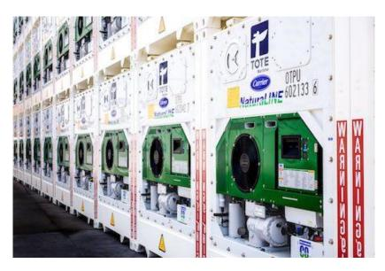
TOTE Maritime Puerto Rico's latest investment in green technologies is the addition of 220 containers leased from SeaCube Containers and refrigerated by Carrier Transicold NaturaLINE units, which use the natural refrigerant carbon dioxide, with an ultra-low global warming potential.
